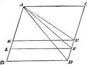
Complete the parallelogram ACDB. Draw AD. Then we have to show that AD represents in *direction* the resultant.
